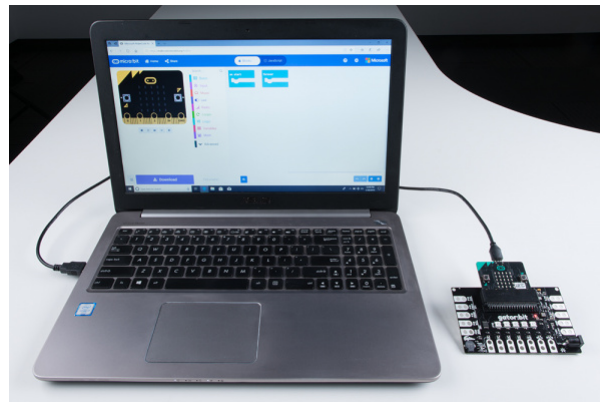
A micro:bit connected to a laptop with a USB cable.
