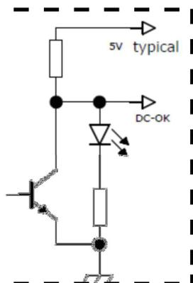
During normal operation, this signal is logic HIGH for output more than 85% (typical) of normal. Signal will go LOW for output less than 80% (typical) of normal. Green LED will light on PCB top side during normal operation
