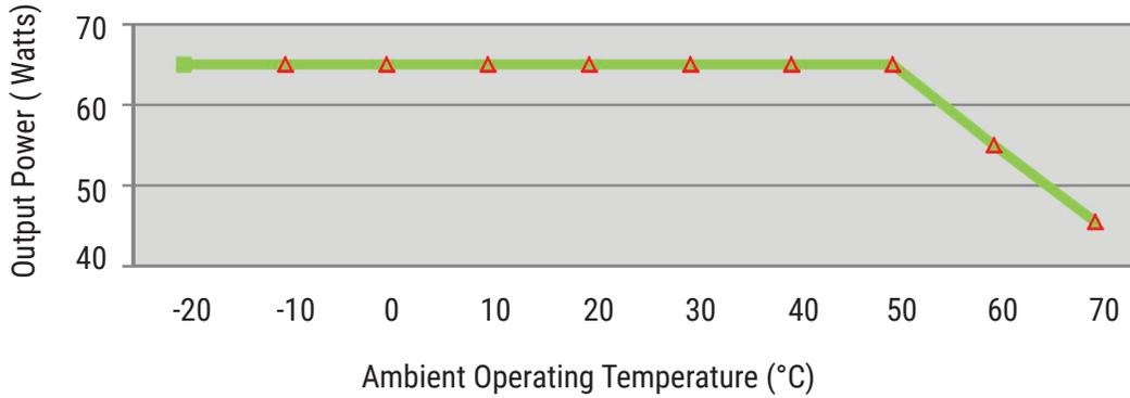
65W convection cooled at -20°C to 50°C operating ambient temperature. De-rated output power to 45.5W at 70°C.
