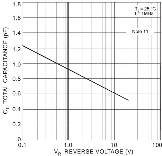
Fig. 3 Typical Total Capacitance vs. Reverse Voltage
