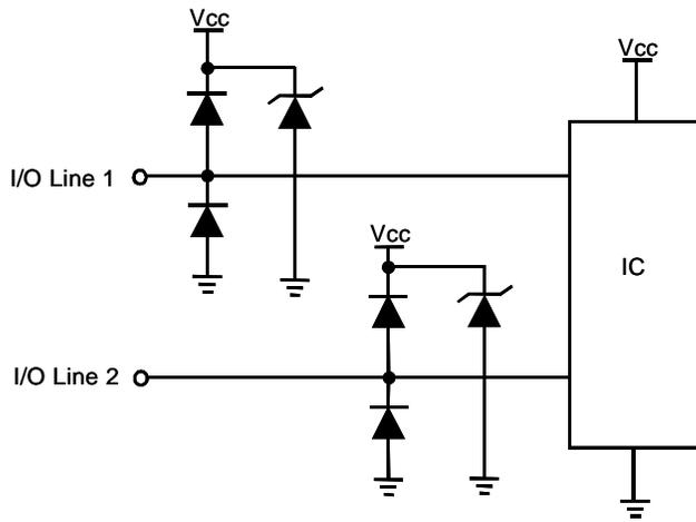
Fig. 6 Data Line Protection
