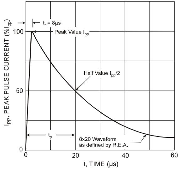
Fig. 2 Pulse Waveform
