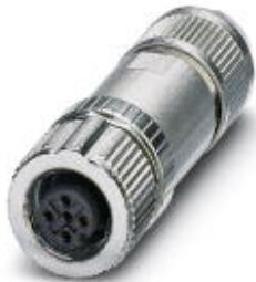
Bus system connector, socket, straight, 5-pos., M12 SPEEDCON, shielded, A-coded, spring-cage connection, metal knurl, cable diameter max. 8 mm
