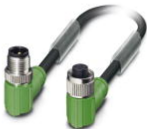
Sensor/actuator cable, 5-position, Variable cable type, shielded, Plug angled M12, A-coded, on Socket angled M12, A-coded, cable length: Free input (0.2 ... 40.0 m)
