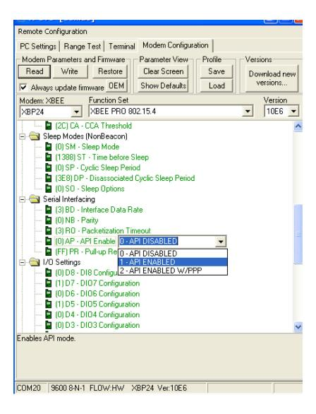
**Note:** To configure parameters on a remote radio, set AP = 1 on your base radio. For more information about the different AP settings, see the API section of the product manual.
