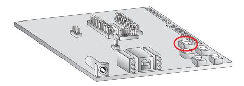
Pressing this button power cycles the module, but will not clear any changes written to the module. This is useful if you are having issues accessing the COM port. This will also reset any parameters that were changed but not written into memory.
