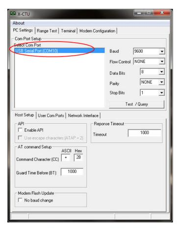
3. Verify that the baud rate and data settings match the internal settings of the devices:
