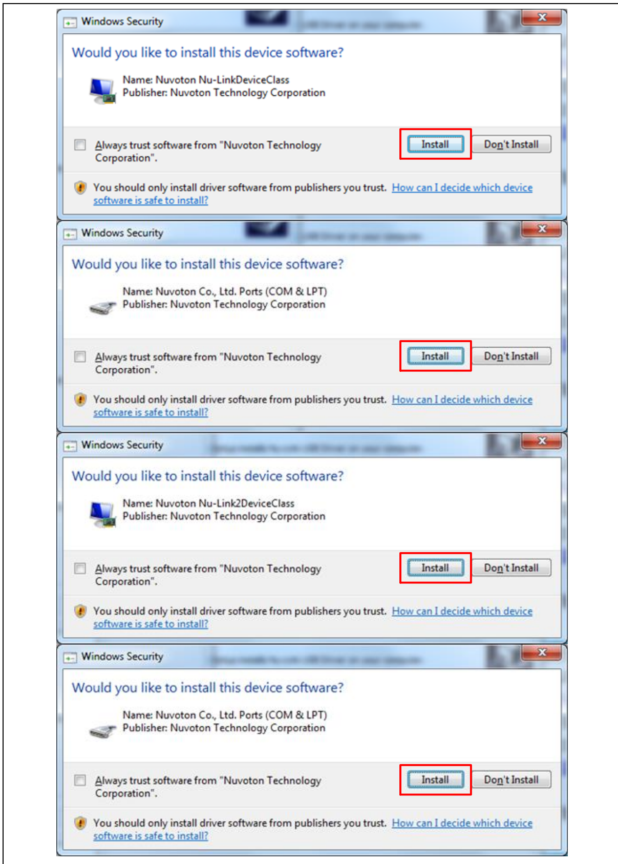
Figure 4-2 Nu-Link USB Driver Installation
