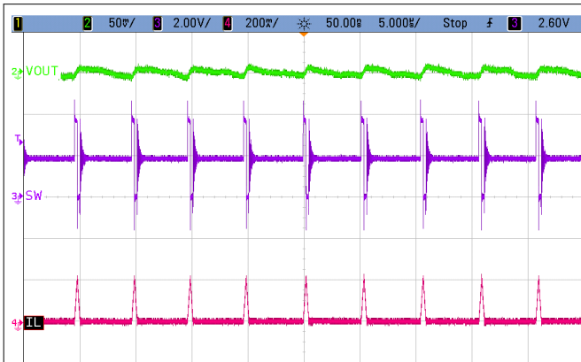
Figure 9-14. PFM (Power Save Mode) Mode Operation
