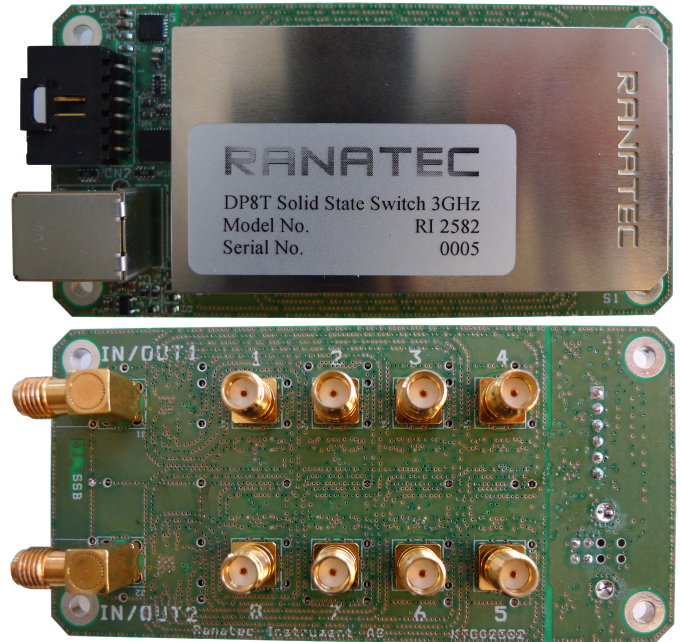
Ranatec RI 2582 is a high performance DP8T solid state switch module suitable for high volume switching applications.
