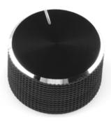
Knobs are a great way to finish off your project and make it easier to adjust the level of your death ray. This knob mates to a 6mm (+/- 0.3mm) shaft. The knob slides onto the potentiometer and holds tightly with a strong friction fit.
