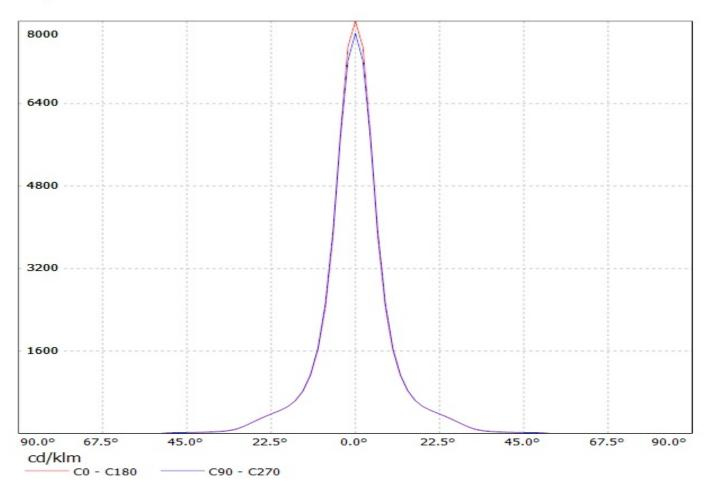
Luminaire: Ledil Oy CA12107\_Lena-S-Diffuser-Lens\_CXA20 CA12107\_Lena-S-Diffuser-Lens\_CXA20
