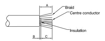
2) Tin the centre conductor. Slide the clamp nut, washer and grommet over the cable. Place the taper clamp over the braid and push back against the cable jacket. Pull the braid back over the taper clamp and trim level with the rear as shown.
