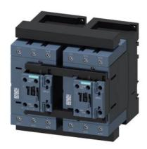
Reversing contactor assembly, AC-3, 37 kW 400 V, 230 V AC/50/60 Hz 3-pole, Size S3 screw terminal electrical and mechanical interlock 2 NO integrated
