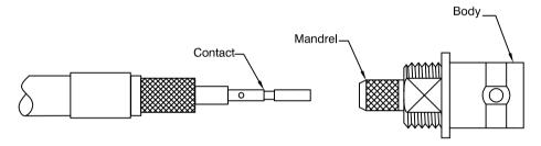
3) Insert the contact into the body and ensure that the contact captivates. Make sure the braid is on the outside of the mandrel. Slide the ferrule over the braid until the ferrule butts up against the body. Crimp the ferrule using the correct tool for the connector.
