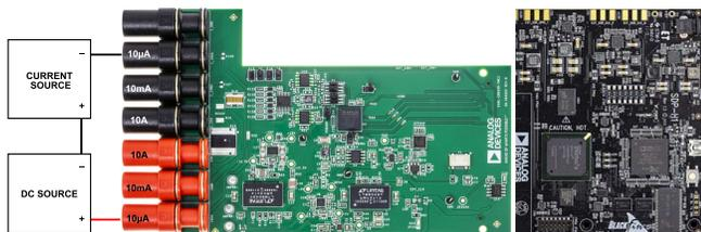
Figure 2. Simplified Evaluation Test Setup, 10  $\mu$ A Range
