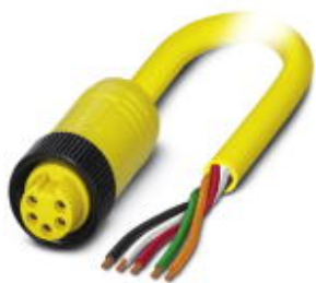
Power cable, 5-position, PVC, yellow, free cable end, A - standard, on Socket straight 7/8"-16UNF, cable length: 1 m
