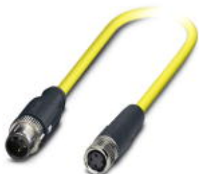
Sensor/Actuator cable, 3-position, PVC, yellow, shielded, Plug straight M12 SPEEDCON, A-coded, on Socket straight M8, Cable length: 1.5 m
