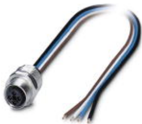
Flush-type connector, Power, 4-position, Socket, M12, T power, Front mounting, M16 x 1.5, Individual wires, cable length: 0.5 m
