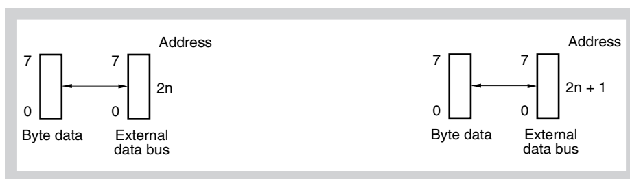
Figure 7-21 Left: Access to even address (2n) Right: Access to odd address (2n + 1)
