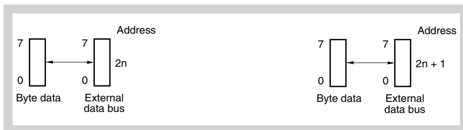
Figure 7-22 Left: Access to even address (2n) Right: Access to odd address (2n + 1)
