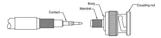
3) Insert the contact into the body and ensure that the contact seated. Make sure that the braid is on the outside of the mandrel. Slide the ferrule over the braid until the ferrule butts up against the body. Crimp the ferrule using the correct tool for the connector.
