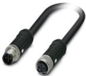
Sensor/actuator cable, 5-position, PE-X halogen-free, black, shielded, Plug straight M12 SPEEDCON, A-coded, on Socket straight M12 SPEEDCON, A-coded, cable length: 5 m, For railway applications
