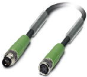
Sensor/actuator cable, 4-position, PUR halogen-free, black-gray RAL 7021, shielded, Plug straight M8, on Socket straight M8, cable length: 3 m
