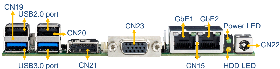
Figure 4.7 UTC-520CU Connector Locations (Coastline)
