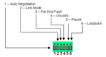
**Note:** All switch changes take effect immediately and will result in a link reset on both ports.
