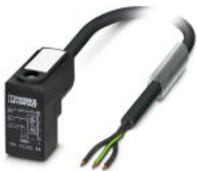
Sensor/actuator cable, 3-position, PUR halogen-free, black-gray RAL 7021, free cable end, on Valve connector C (8 mm), with 1 LED, connected with Z diode, cable length: 5 m
