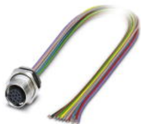
Sensor/actuator flush-type socket, 12-pos., M12 SPEEDCON, rear/screw mounting with Pg9 thread, with 0.5 m halogen-free TPE litz wire, 12 x 0.14 mm 2
