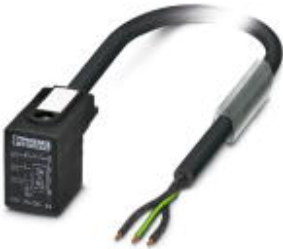
Sensor/Actuator cable, 3-position, PUR halogen-free, Black-gray RAL 7021, Free cable end, on BI valve plug (11 mm), with 1 LED, connected with Z diode, Cable length: 5 m
