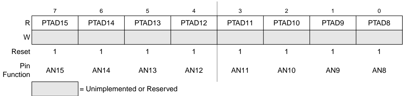
Figure 7-16. Port Data Register 0 (PORTAD0)
