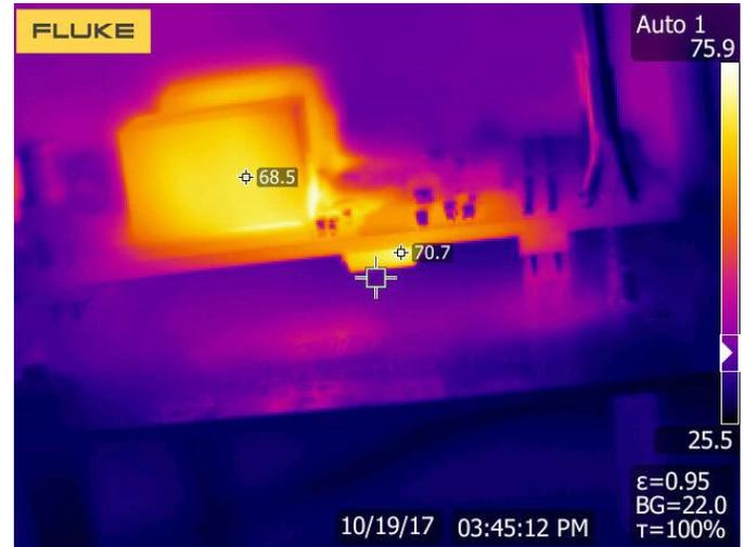
**Figure 19: Thermal image of the LSICRD-GD-ISO5852 with ISO5852S and 2 Ohm gate resistance operating at 200 kHz**
