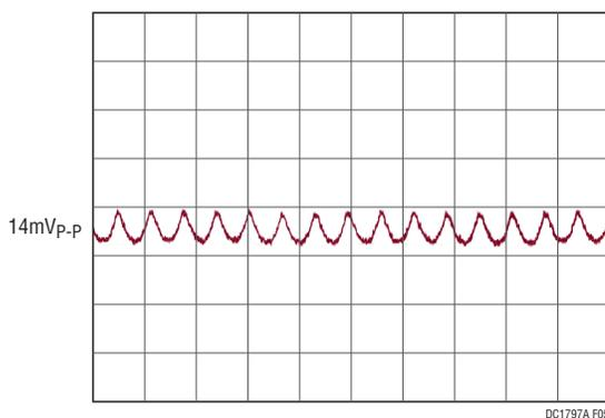
**Figure 5. Output Noise, V<sub>IN</sub> = 4.5V, I<sub>OUT</sub> = 1A**
