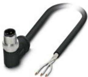
Sensor/Actuator cable, 3-position, PE-X halogen-free, black, shielded, Plug angled M12 SPEEDCON, A-coded, on free cable end, Cable length: 2 m, For railway applications
