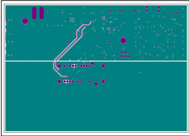
Figure 10. Board layout—power plane, Layer 3.
