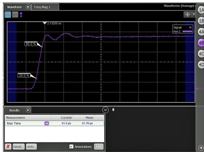
Figure 4: PV1 step response, measured with an 8-picosecond stimulus source
