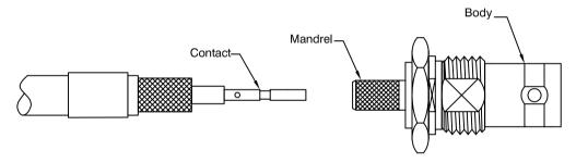
3) Insert the contact into the body and ensure that the contact captivates. Make sure that the braid is on the outside of the mandrel. Slide the ferrule over the braid until the ferrule butts up against the body. Crimp the ferrule using the correct tool for the connector.
