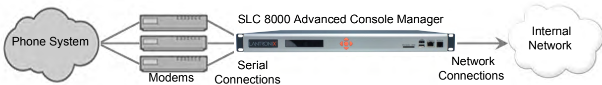
Figure 11-2 Remote Access Server
