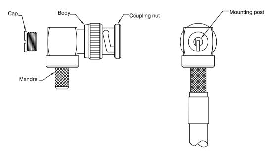
3) Slide the ferrule over the braid until the ferrule butts up against the body Crimp the ferrule using the correct tool for the connector. Solder the center conductor to the mounting post and fit the end cap in place.
