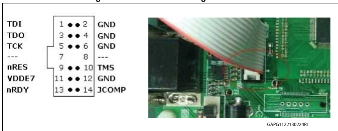
Figure 8. JTAG / Nexus debug connection
