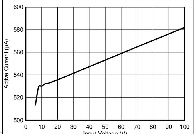
Figure 6.  $V_{IN}$  Active Current versus Input Voltage
