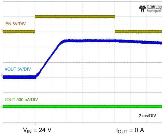
Figure 19. No-Load Start-up and Shutdown with EN/UVLO
