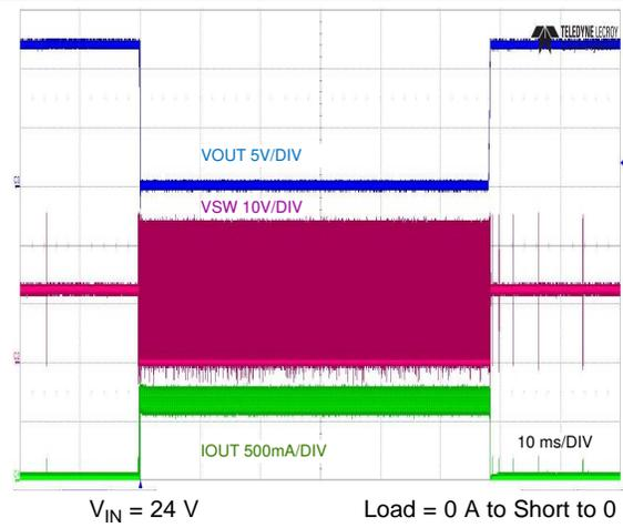
Figure 24. No Load to Short Circuit/Short Circuit Recovery
