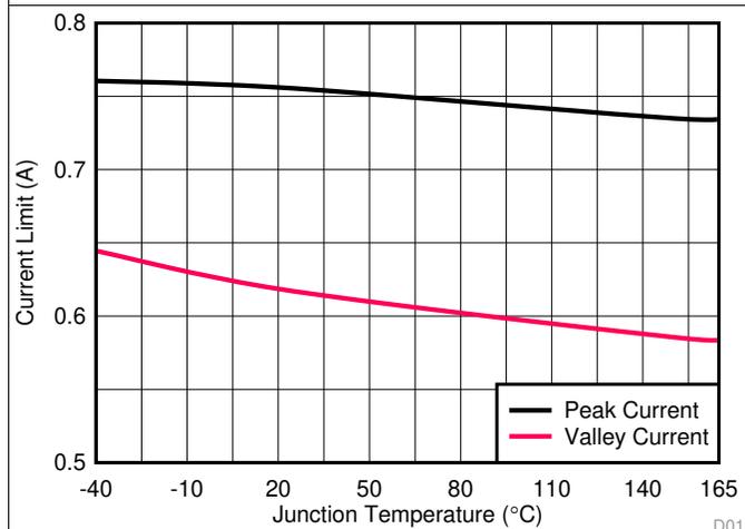
Figure 9. Peak and Valley Current Limit versus Temperature
