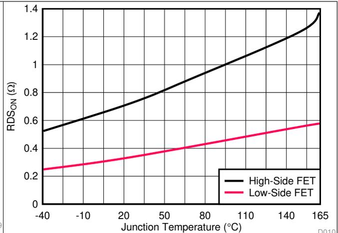
Figure 8. MOSFETs On-State Resistance versus Temperature
