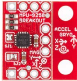
The MPU-9250 Breakout as you will receive it
