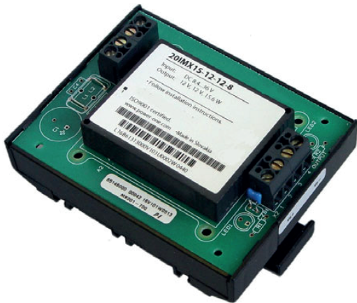
Fig. 24 DIN-rail mounting support DMBIMX15 (HZZ00625)
