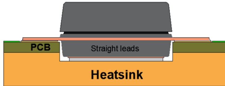
Figure 3. PCB bonded to a heat sink with a cavity, intended for straight leads package
