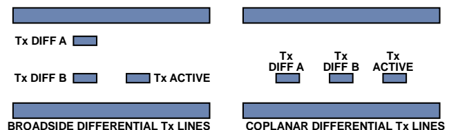
Figure 66. Broadside vs. Coplanar Differential Stripline Routing Techniques
