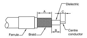
2) Crimp the contact onto the centre conductor.
