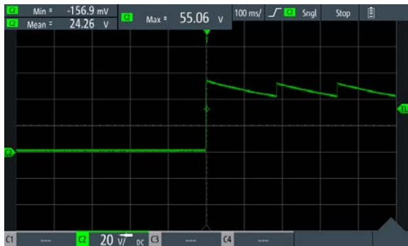
Figure 9. Turn-On Transient at a Time Scale of 100 ms
