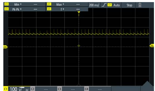
Figure 11. Hysteretic Regulation Measured at C11 at a Time Scale of 200 ms
