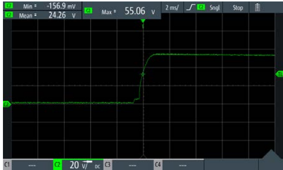
Figure 8. Turn-On Transient at a Time Scale of 2 ms
