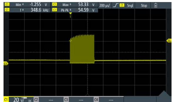
Figure 12. Boost Pulses at MOSFET Q2 Drain Terminal at a Time Scale of 200 μs
