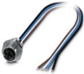
Flush-type connector, Power, 4-position, Socket, M12, T power, Front mounting, M16 x 1.5, Individual wires, cable length: 0.5 m
