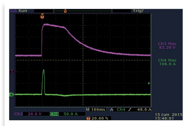
Figure 13: 24V system 10pulses by 202V, 350mS, 1 ohm R_i with 5 SLD10-018 connected in series
