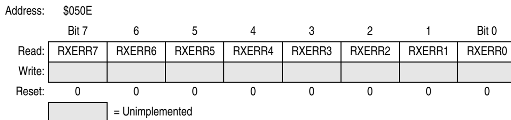
Figure 12-25. Receiver Error Counter (CRXERR)
