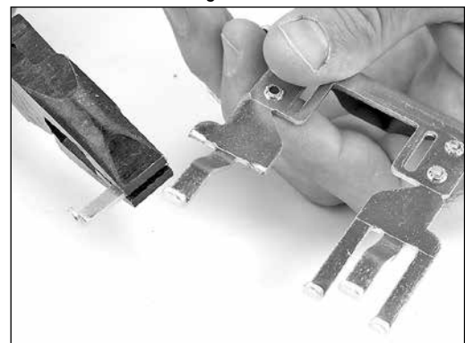
Figure 20: Prongs being broken off
