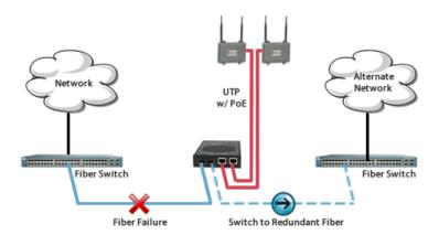
2. **Redundant Primary**: When the primary link fails, the media converter redirects traffic to the secondary fiber port within 50ms. Upon restoration of the primary fiber link, traffic is automatically redirected back to the primary fiber.
