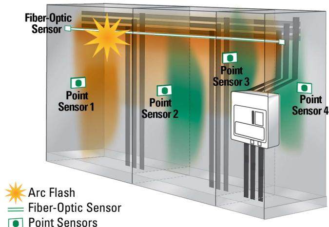
Scenario with point sensor placement on the wall of each compartment. Arc detection area for each sensor is shown in green shade. In this case, both Point Sensor 1 and the Fiber-Optic Sensor detected the flash as it was within their viewing area (shown in orange).
