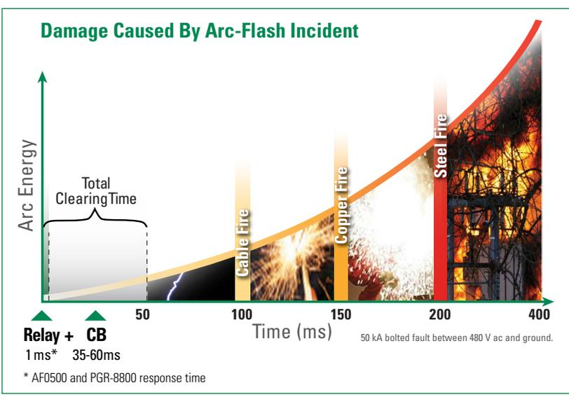
The Littelfuse Arc-Flash Relays use a 125- $\mu$ s light-sampling scheme in combination with an ultra-fast IGBT output to be able to detect a developing arc flash and send a trip signal to a circuit breaker in milliseconds.
